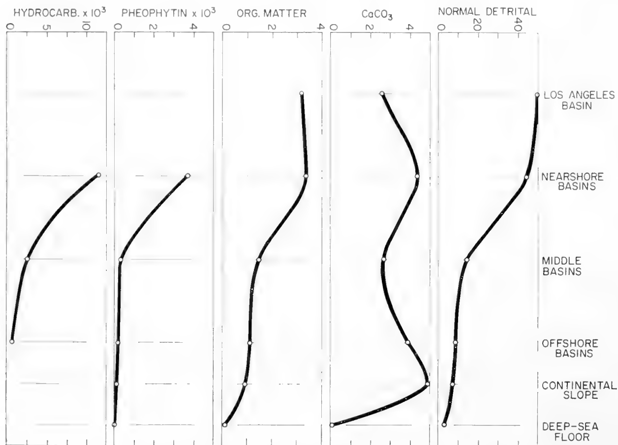
Fig. 3. Curves showing rates of accumulation of various components of southern California basin sediments. Note the similarities and differences between curves for absolute rates of deposition and for the percentage compositions given in Fig. 2. Values for organic matter are at the surface of the sediment. (From Emery, 1960, fig. 208.)
